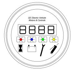
The FSIP Standard Dash Display is a four segment Light Emitting Diode (LED) instrument that displays the FSIP LX, ZX, and SX Status Codes, Hourmeter Readings, Battery Discharge Indication, and Maintenance Required Code. The four LED's above the symbols indicate the active readout mode.
