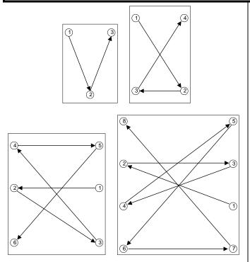
Proper sequence for use in tightening hardware during control mounting
